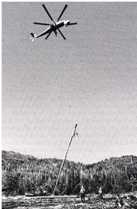
Fig. 12. Modern yarding of logs with a helicopter in California. [Courtesy U.S. Forest Service.]
