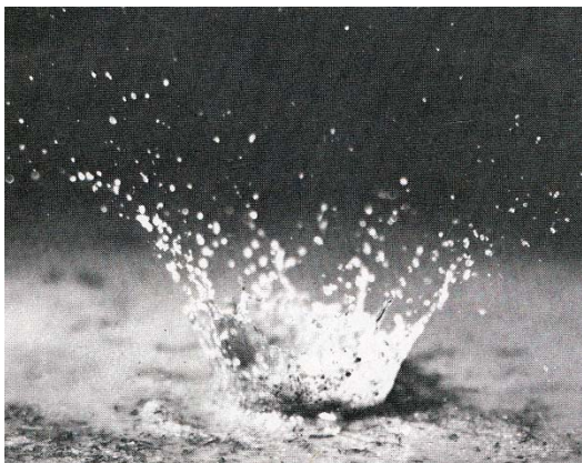
Fig. 12. A stroboscopic photograph has caught the impact of a raindrop on moist soil, bursting upward and outward and carrying soil with it. [Courtesy USDA.]
