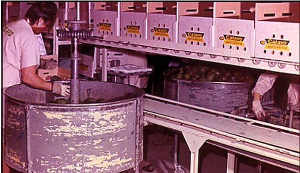
Layers of fruit are placed on top of styrofoam liners and when full are pushed onto the conveyer belt shown to the right of the tub
