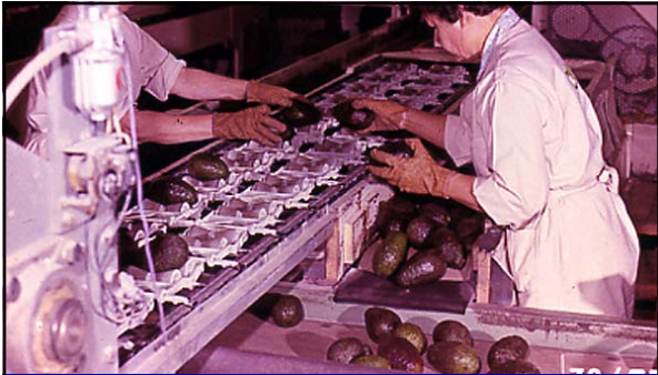
After the fruit is graded it is placed in cups ahead of the stamping machine which places the packing house trade name on the fruit
