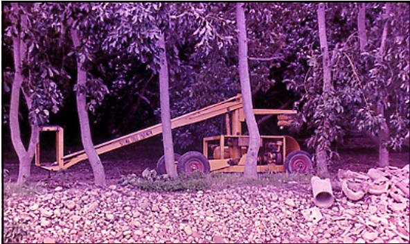
The Selma Tree Farmer is a mechanical aid for pruning or harvesting of fruit
