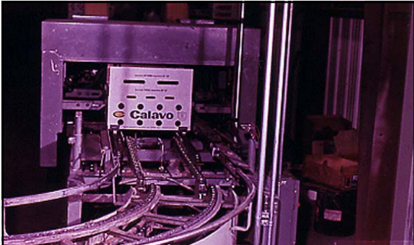
Boxes pass into this machine which automatically applies glue and folds down the flaps holding them for a sufficient time for the glue to set
