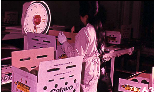
Each carton passes this weighing station where the total weight is adjusted to a uniform total weight by either adding or taking away of fruit
