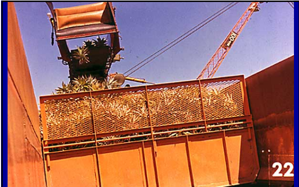
A large special truck just ahead of the conveyer is equipped with a movable front end enclosure
