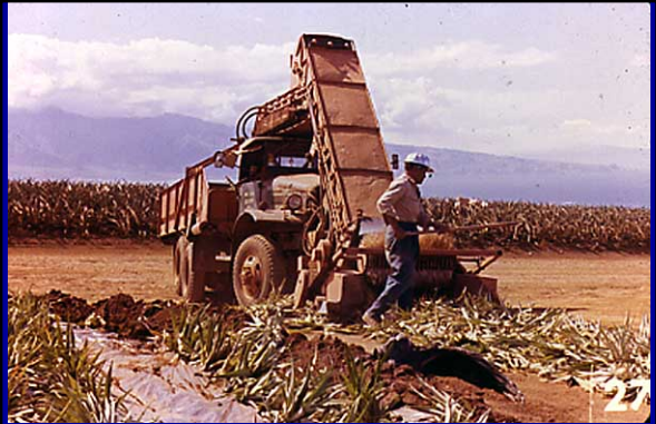
Surplus plants are placed in the drive rows and picked up by the conveyer on this truck
