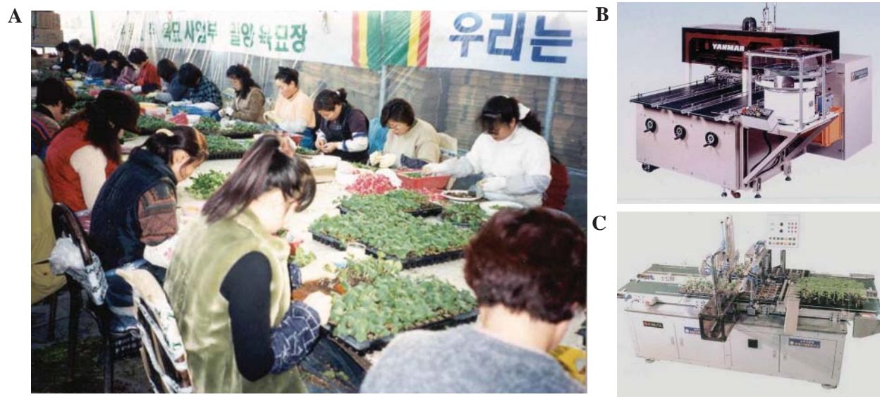
Fig. 12-18. Grafting vegetables. A. Manual grafting in Korea. B and C. Korean and Japanese machines developed for grafting (Lee and Oda, 2003).
