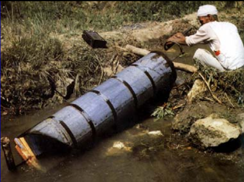
An Egyptian farmer turning an Archimedes screw by hand to irrigate a field
